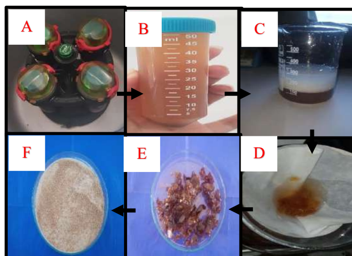
Figure 1: Purification of an Adjuvant used for the formulation of botanical insecticide; (A)- Centrifugation, (B)- Polysaccharide solution, (C)- Precipitation, (D)- Washing, (E)- Drying, (F)- Grinding
